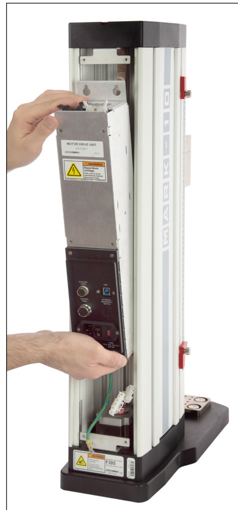
Removing the MDU
