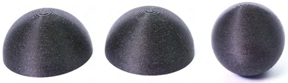
Pict. 29 - A sphere printed in two separate parts glued together
