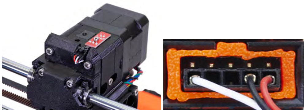
Pict. 38 - Properly connected and seated filament sensor
