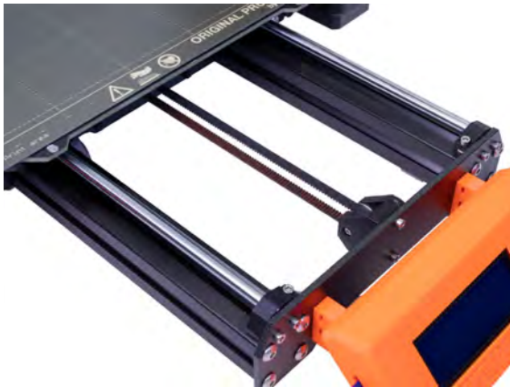
Pict. 47 - A properly-tightened Y-axis belt under the heatbed
