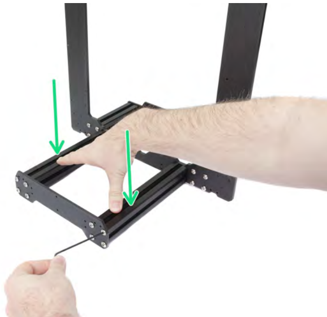
Pict. 45 - Proper way to tighten the frame, plates and aluminum extrusion together.
