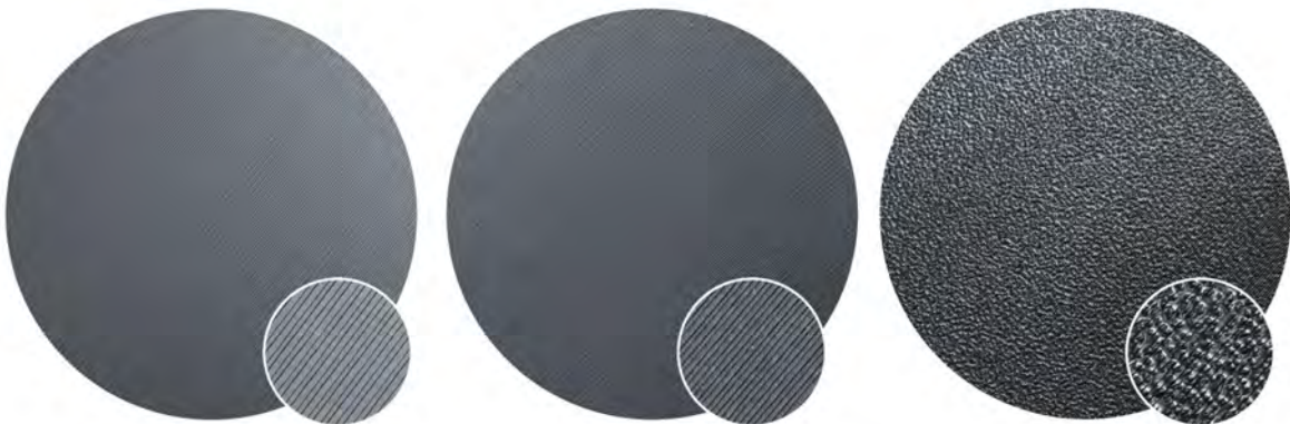
Pict. 7 - Smooth PEI sheet (left), Satin powder coated sheet (middle), textured powder coated PEI sheet (right) effect on the first layer
