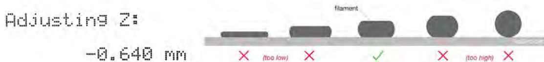
Pict. 10 - How to tune the nozzle height live during the test print. Note: -0.640 mm is only for illustration. Your setting will be different!
