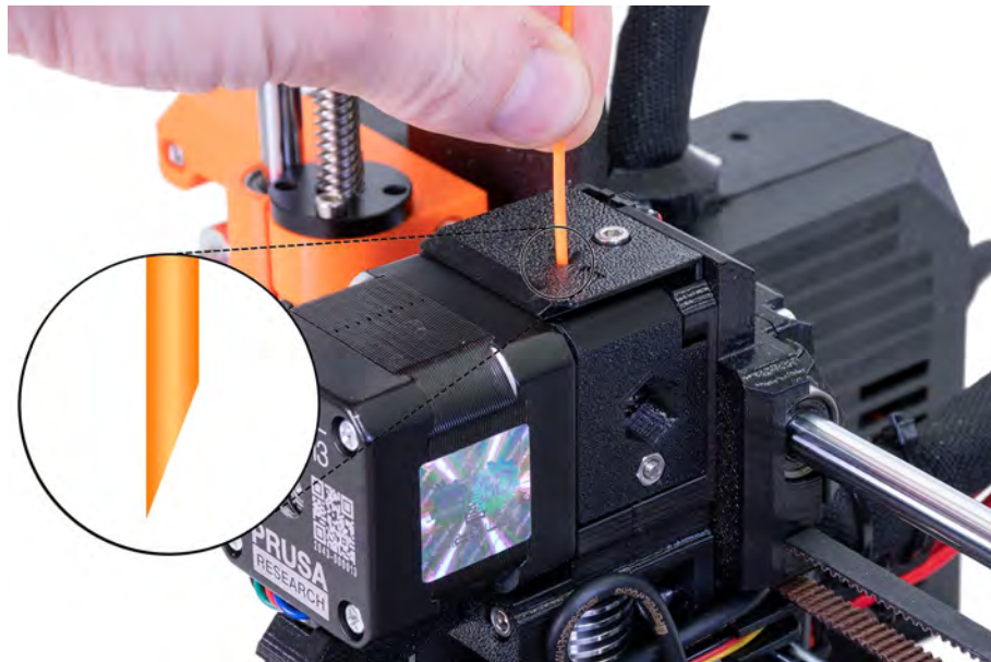
Pict. 9 - Loading the filament into the extruder
