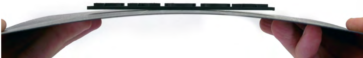
Pict. 13 - Removing the model from the PEI print surface by bending the steel sheet.
