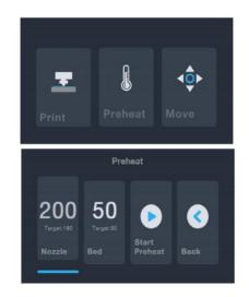
9. Touch the Start Preheat button to start preheating the nozzle and build plate. Once the target temperatures are reached, the button will change to Stop Preheat and the displayed nozzle and bed temperatures should be at or near your target values. 10. While the printer is heating, open your filament. Using a pair of scissors or side cutters, diagonally snip the end of the filament to make a point, as shown in the images below.
