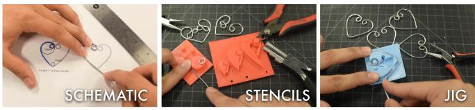
Figure 1. a) Schematic, an annotated construction proxy used to provide fabrication feedback, b) Stencil, a fabrication proxy that breaks down designs into elementary forms, c) Jig, a fabrication and construction proxy that provides a ritual high-fidelity fabrication process.
