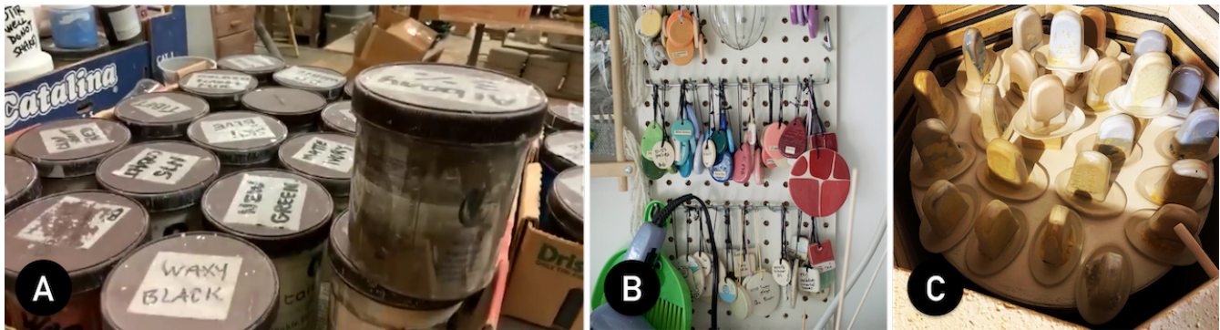
Figure 1: A) A ceramics instructor labels personal time-tested glazes for her studio, B) a production ceramicist hangs a collection of glaze keys that allow her reference and share her glaze and clay body combinations with others in her communal studio; C) a ceramics engineer systematically fires variations of a glaze recipe for documentation and analysis.
