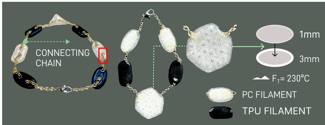
Figure 13: Thermoplastics as a Precious Material. A. An initial TackFuseTechnique of gold chains onto thermoplastic gems, B. a PC ‘geode’ is Microslumped using a triangle infill and EncapsulatedFused to gold chains to form a necklace, C. FirePolishedTechnique thermoplastic gems.
