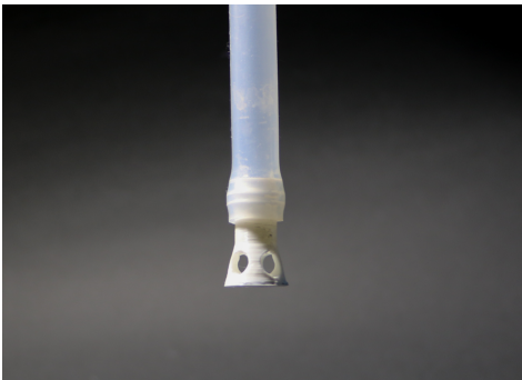
Figure 3: Drainage Tube Adaptor to prevent artifact deformation
