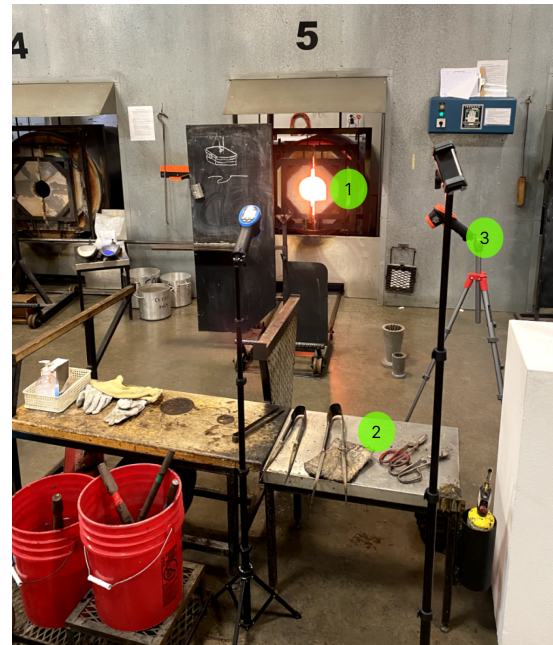
Figure 3: To capture the data necessary to train our ShatterModel, we used a setup of two cameras and two pyrometers each capturing different angles of the glass. The glass shop forms an adverse environment for technology: (1) the furnace operates in temperatures well outside technology operating ranges; (2) the tools and workbench change their position daily; (3) every space is critical to glassblowing – with just a few cameras and pyrometers set up, much of the usable space is taken up.
