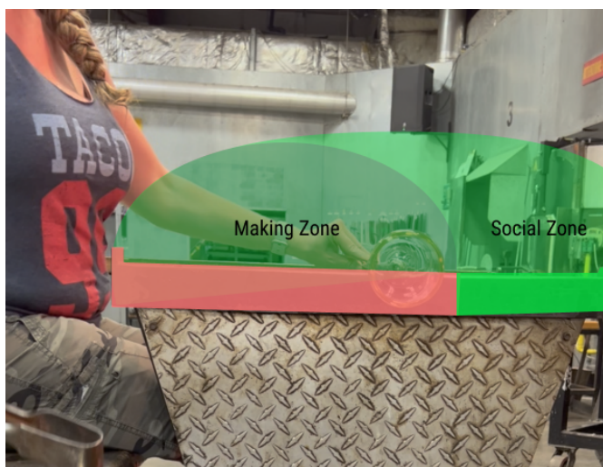
Figure 4: The glassblower uses the rail to support their blowpipe while rotating their piece. The rail can be split into two areas of spatial interaction, a making zone and a social zone. The making zone houses the majority of rotations, while the social zone is often used to communicate with the assistant.
