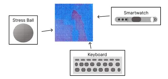
Figure 1: The Pits Texture. The Pits texture, made from cast silicone, features depression geometries of 0.53 mm by 0.5 mm and a spacing of 1.06 mm apart. A tap gesture was one of the preferred methods of stimulation, for which it was perceived as smooth, soft, silky, and fuzzy. Value could be found in applications such as wearable devices, haptic devices, and sensory devices.
