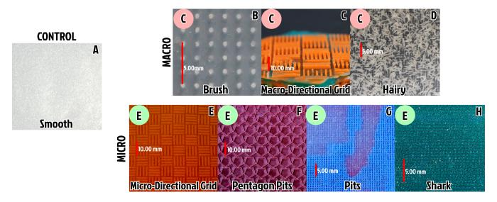
Figure 2: Castura Fabricated User Study Textures. A selection of textures that were fabricated via the *Castura* method. Textures marked with a "C" were fabricated with cut plates, while textures marked with an "E" were fabricated with an etched plate.
